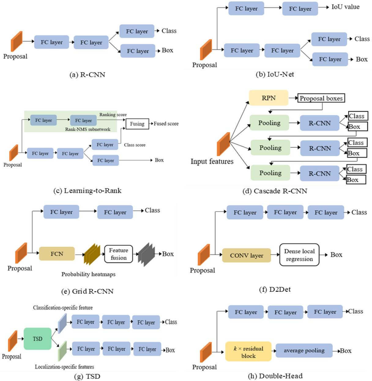
**Figure 11.** The structure of the detection head: (a) R-CNN; (b) IoU-Net; (c) Learning-to-Rank; (d) Cascade R-CNN; (e) Grid R-CNN; (f) D2Det; (g) TSD; (h) Double-Head
