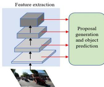
**Figure 4.** Object detection based on multi-layer features [20-22]
