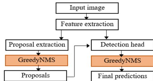
Figure 12. Faster R-CNN with GreedyNMS as a post-processing stage
