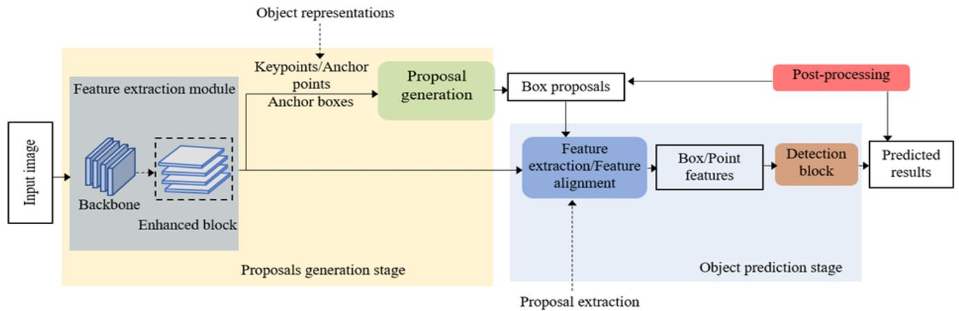
**Figure 2.** The structure of two-stage object detection framework
