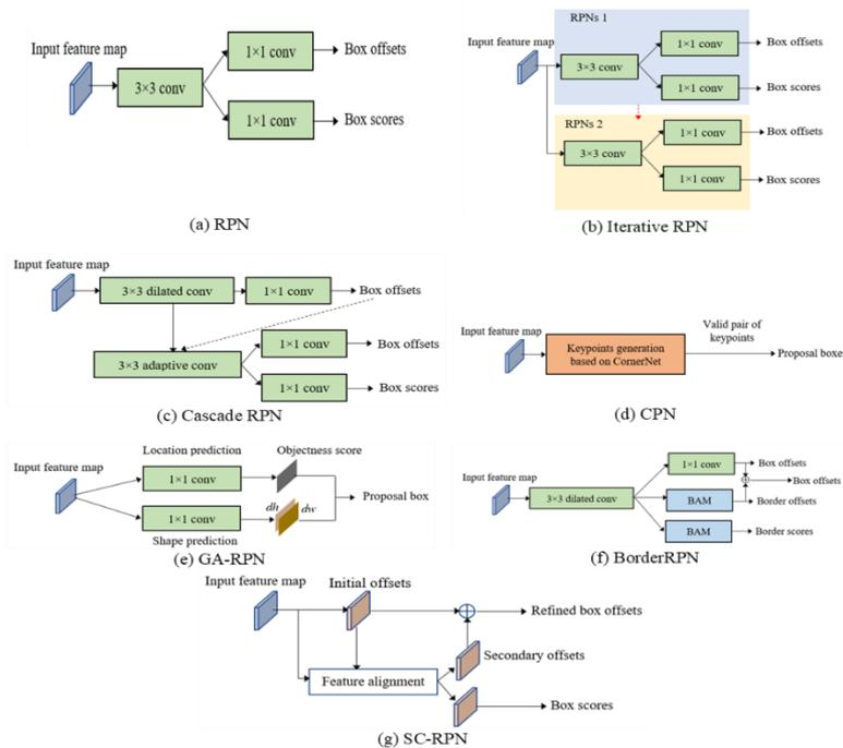
**Figure 9.** The structure of proposal generation networks: (a) RPN; (b) Iterative RPN; (c) Cascade RPN; (d) BorderRPN; (e) CPN; (f) GA-RPN; (g) SC-RPN
