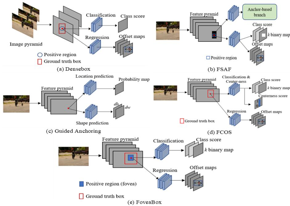
**Figure 6.** Object detection based on anchor-point representations: (a) Densebox; (b) FSAF; (c) Guided Anchoring; (d) FCOS; (e) FoveaBox
