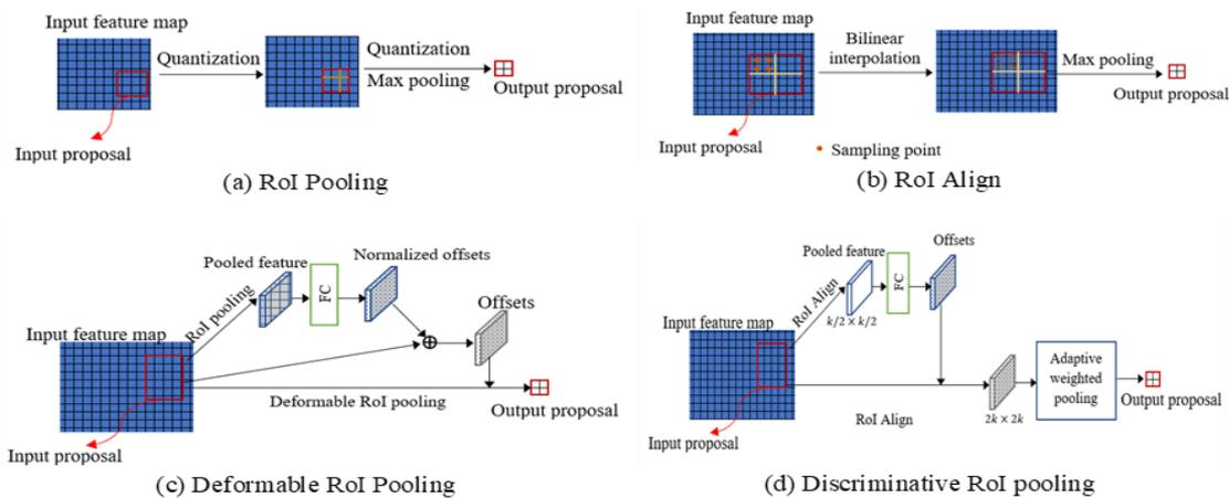
**Figure 10.** Proposal extraction methods: (a) RoI Pooling; (b) RoI Align; (c) Deformable RoI Pooling; (d) Discriminative RoI pooling
