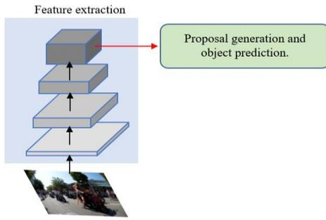
**Figure 3.** Object detection based on a single-level feature map [30, 52]
