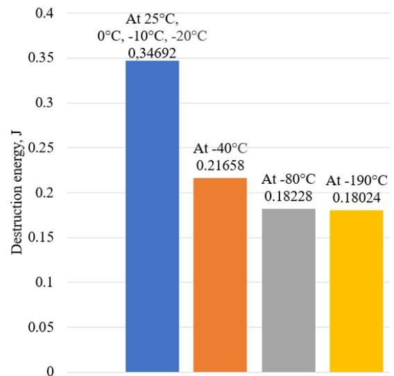
**Figure 4.** Impact strength for samples with an average diameter of 10 mm at various temperatures
