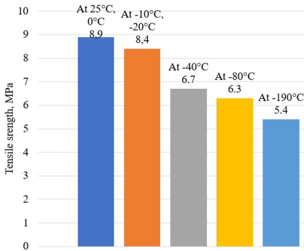
**Figure 2.** Compressive strength values for samples with an average diameter of 10 mm at different shell temperatures
