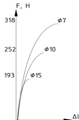
Figure 1. Compression of samples with various average diameters
